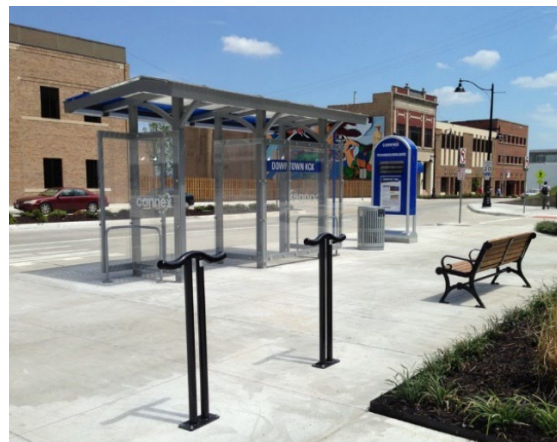
Figure 7: Bus stop with large accessible pad, seating, shelter, and integrated active transportation, Kansas City
