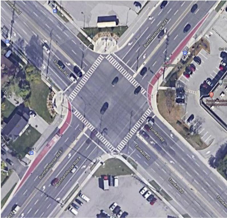
An ideal configuration will require a right of way of approximately 45m in length, and 3.5m in width on the far-side of the intersection, inclusive of the merging space back into mixed traffic. If the full right of way requirement is not available, alternative configurations may be considered including:
