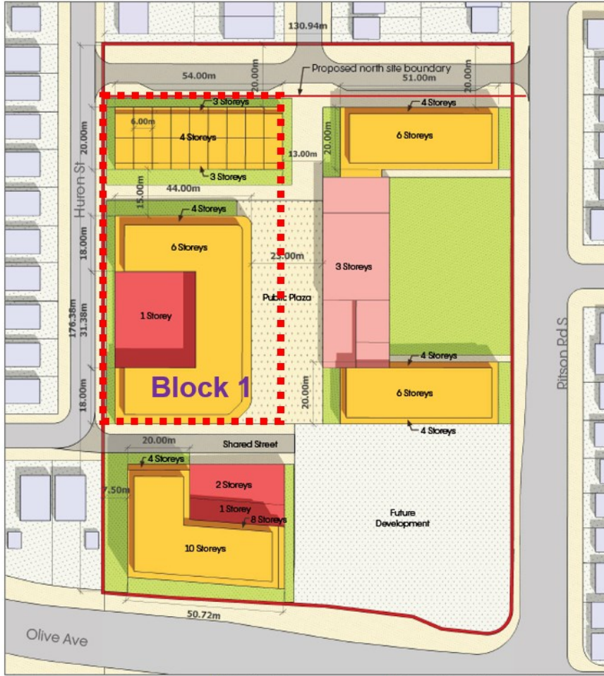
Site Plan ← N Residential Commercial and Community Former Ritson School Public Amenity Space Public Plaza Future Development
