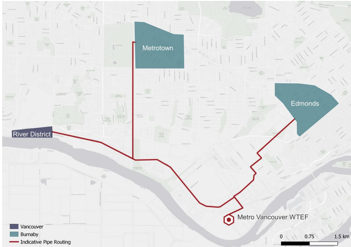
Figure 7: Thermal Energy Transmission Line from WTEF to River District Energy, Metrotown and Edmonds
